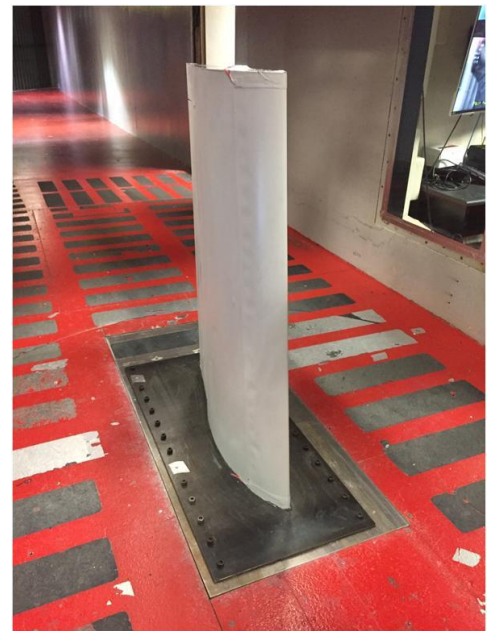
Figure 1: MQ-1 wing test section installed in the IRT tunnel.
