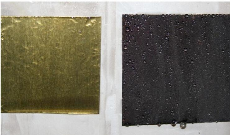
*Filmwise condensation on an untreated brass surface (left) and dropwise condensation on a NEI superhydrophobic brass surface (right)*
